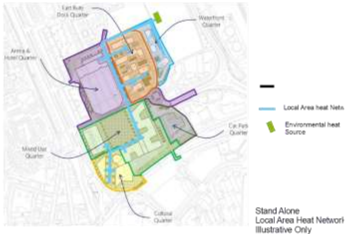
Figure 4-13 Illustration of 5th Generation Ambient Loop as the heat Network solution
